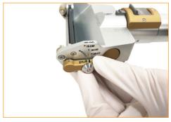
Figure 5. Adjust cutting thickness
